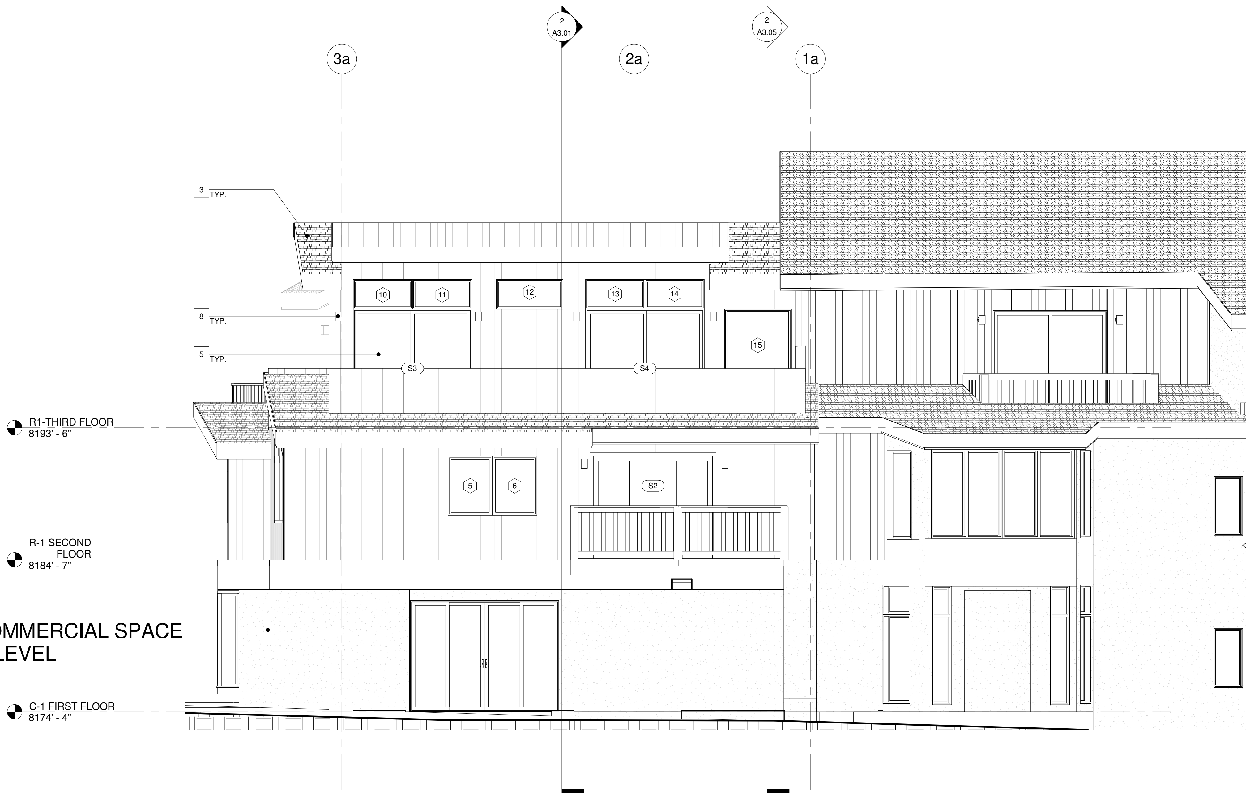
2 EAST ELEVATION - PROPOSED 1/4" = 1'-0"
