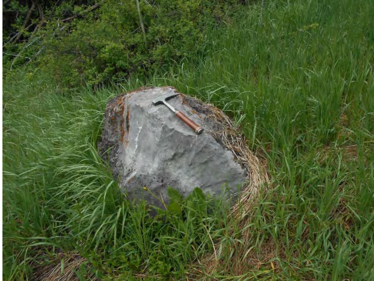
Photograph 19. View of limestone boulder, embedded. Blocky, angular, and about 3 feet in diameter. Boulders like this one are common on the property and are either embedded in the soil (older, ancient rockfall events) or are sitting on top of the soil with minimal soil embedment or vegetation overgrowth.
