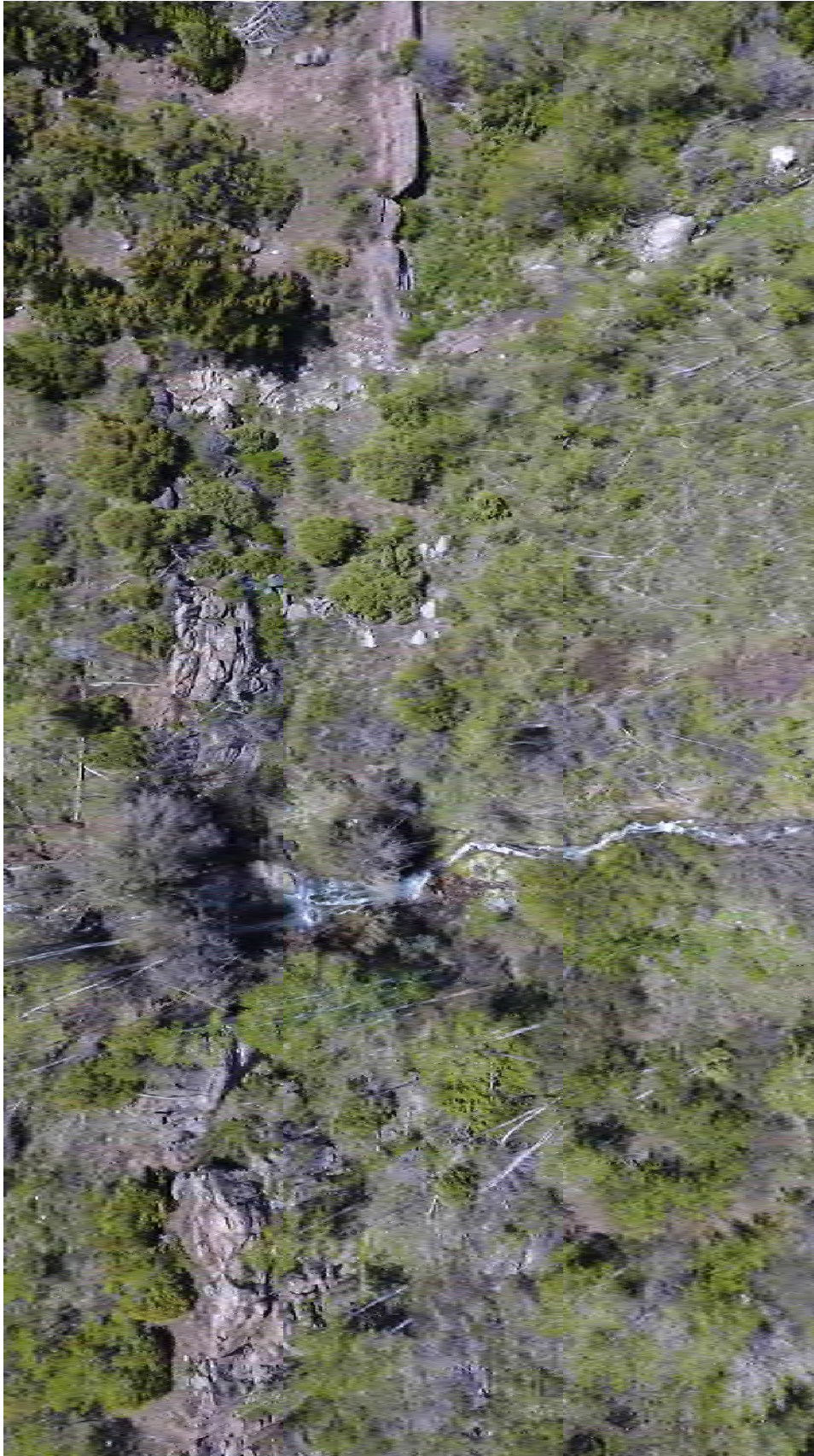
Photograph 18. Aerial view of the rockfall source zone. This photograph shows the steep cliff forming exposures of Robinson Limestone member of the Minturn Formation, dense vegetation in the form of trees and large shrubs, and flowing water in one of the drainages on the west side of the site. The bedrock exposures are fractured, blocky, and ledge-forming.
