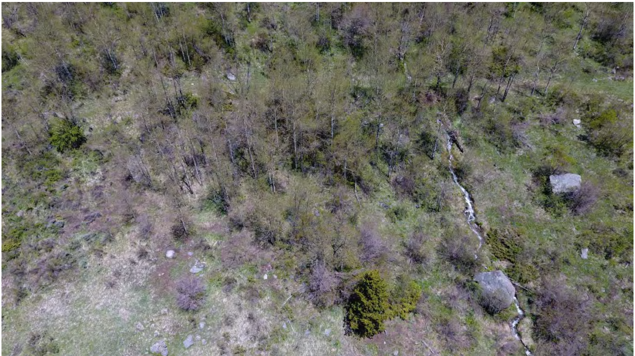
Photograph 23. Aerial view of lower slope in western part of the site. North is toward the top of the photograph. Notice scattered boulders as large as about 7 to 8 feet in longest dimension and slab shaped. Most boulders are 3 feet or less in dimension and are embedded in the soil, representing older, ancient rockfall events.
