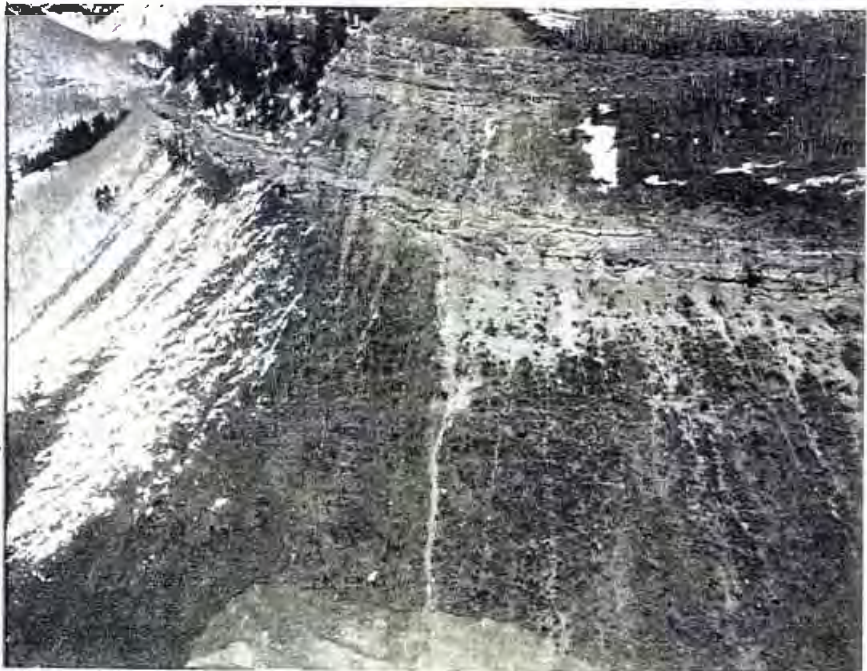
Photo #1. Booth Creek rockfall source area. Note enlargement of upper cliff exposure and corresponding rockfall source area, northwest of the ditch and berm terminus.
