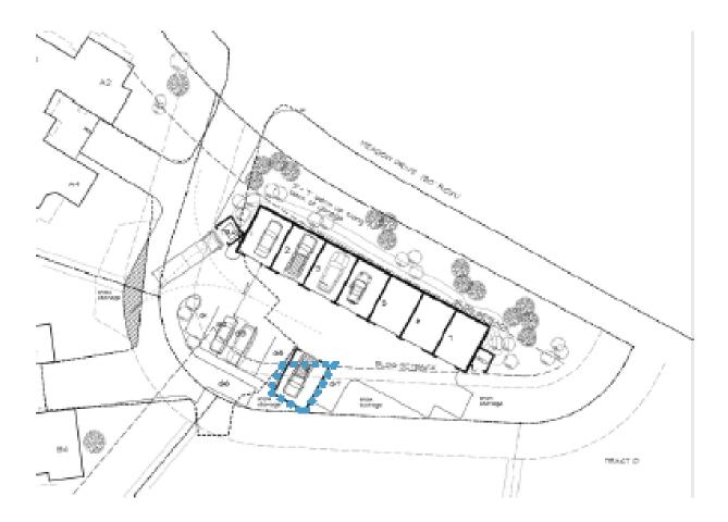
The proposed residential eight (8) unit garage project includes seven (7) garage bays in one structure along Meadow Drive and one standalone unit. All of the garages will be accessed from an internal driveway.
