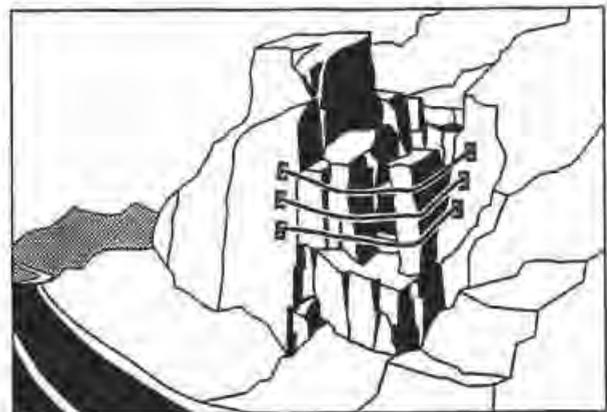
Figure 5. Cable lashing.
