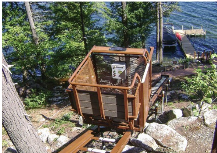
Small funicular providing access from a private residence down to the waterfront.
