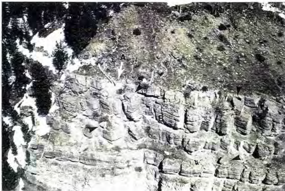
Photo #3. Close-up aerial view of source area. Note ledgy appearance with joint defined blocks undermined by eroding shale partings. White arrow A marks scar from March 26, 1997 rockfall. White arrow B marks rock pedestal that was hit by rockfall and may be destabilized. Note loose blocks, marked by black arrows.
